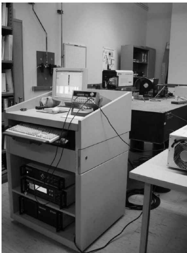
Fig. 3a Experimental setup for laser vibrometry.
